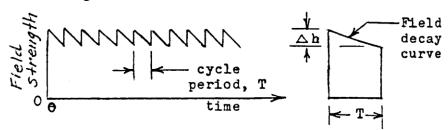
Figure IX-2. Saw-Tooth Waves
