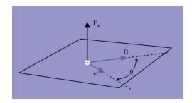
FIG. 29-2. The magnetic force  $F_m$  is perpendicular to the plane of v and B.
