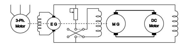
Fig. 12-23 Basic representative circuits of an adjustable-voltage control system.
