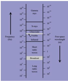
FIG. 35-19. The electromagnetic spectrum.
