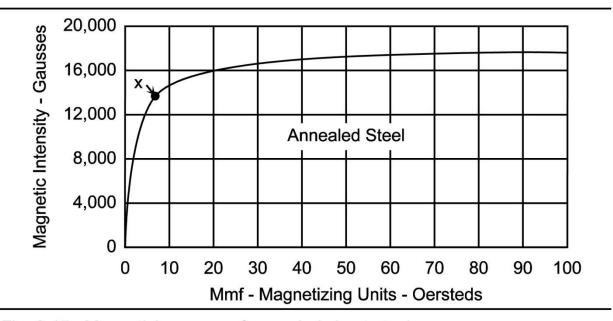
Fig. 8-15 Magnetizing curve of annealed sheet steel.
