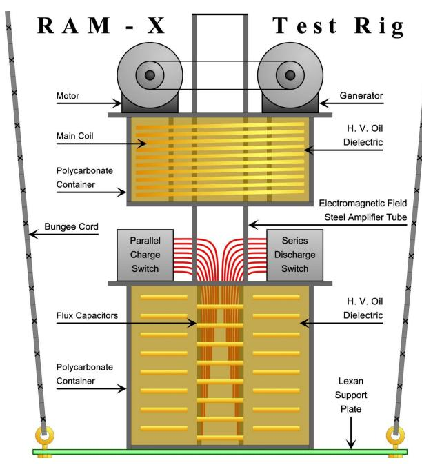
Figure 38 – RAM Test Rig
